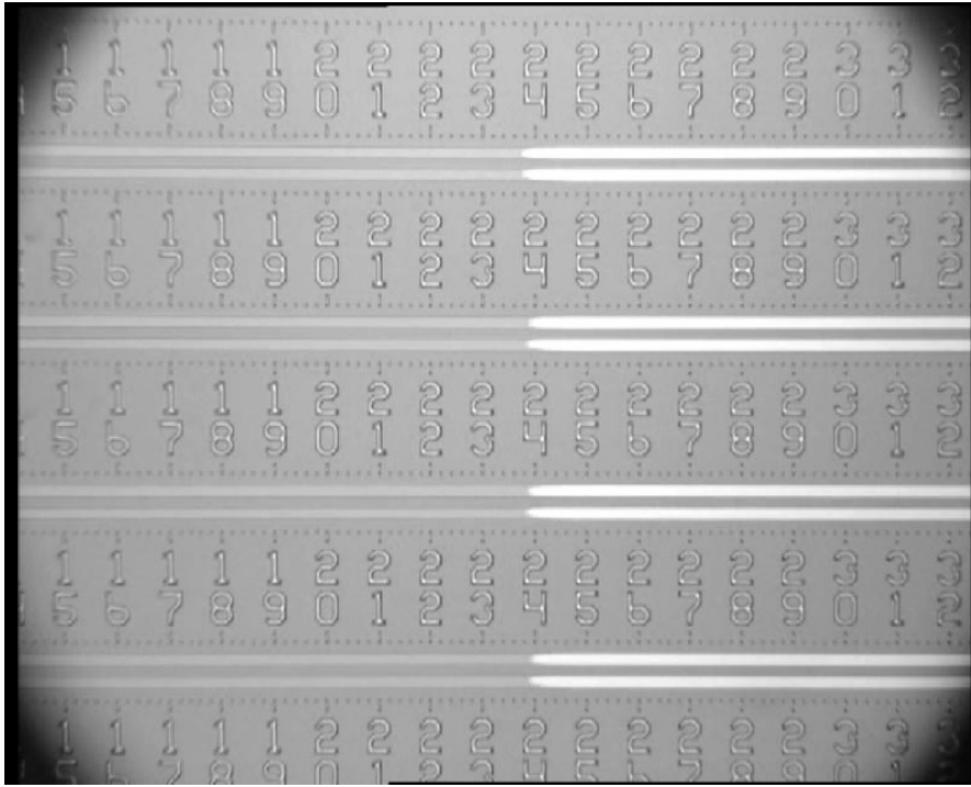
Figure 4-2: A typical still image of the capillary filling of 110 nm deep channels (the large tick marks represent a distance of 100 \mu\text{m} ).
